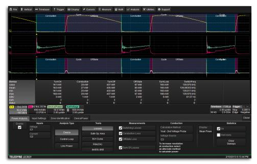
Switching transitions, conduction losses and off-sate losses are color-coded and automatically calculated. Measurements are displayed as energy (joules), mean or peak power (watts). For discontinuous supplies, off-state loss provides an excellent tool to fine adjust a current probe's DC offset and improve measurement accuracy.
