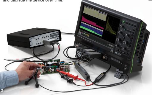
Teledyne LeCroy's HDO4000 and HDO6000 High Definition Oscilloscopes with 12-bit HD4096 technology are the ideal oscilloscope for power measurement. With 16x more resolution than a traditional 8-bit oscilloscope signal details of the saturation voltage are now clearly visible and conduction losses are more accurate.
