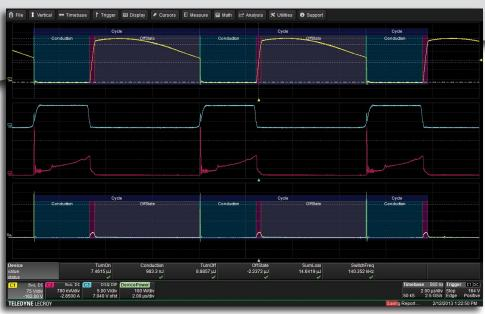
Automatically and accurately analyze the performance of switched-mode power circuits
