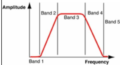
Band-pass filters are useful for emphasizing a selected frequency band. Sample applications include radio channel identification, broadband transmission, ADSL, clock generators (i.e., eliminating the central frequency and displaying harmonics only), and telecommunications (Jitter measurement over a selected frequency range).
