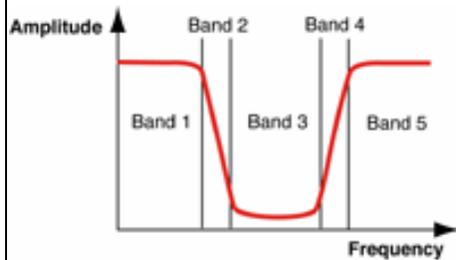
Band-stop filters are useful for eliminating a narrow band of frequencies. Sample applications include medical equipment, such as ECG monitors where the dominant ripple at 50/60 Hz is rejected, leaving the low energy biological signals intact. Digital troubleshooting: the inherent frequency of the switched power supply is blocked, revealing power line voltage drops and glitches caused by the system clock generator.
