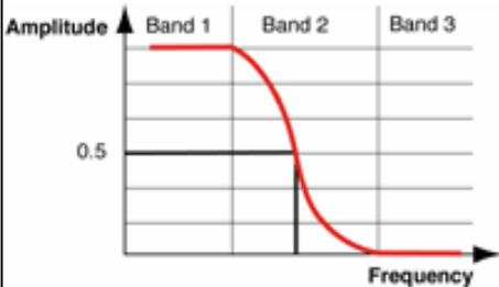
These filters belong to the low-pass filter category (with a variety of shapes). Raised cosine is one of a class of filters used to minimize intersymbol interference: the time domain impulse response crosses zero at all bit time intervals except the one with the impulse.
