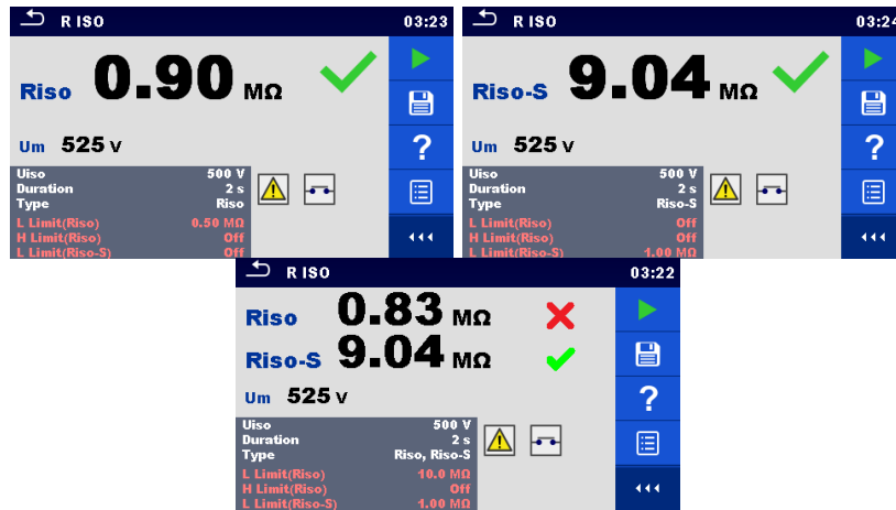
Figure 6.39: Examples of Insulation resistance measurement results
