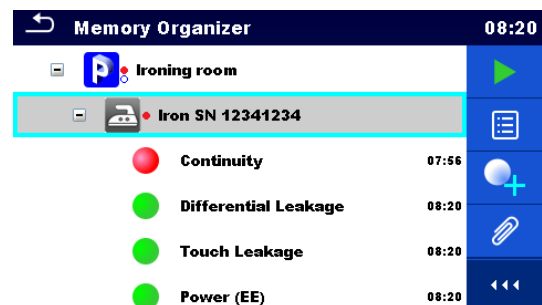
Figure 5.6: Status - Measurements completed with fail result(s)
