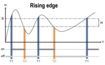
Measurement (m) > Threshold (S) during the time-delay T1  $\rightarrow$  Alarm activation.
