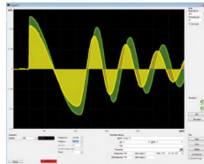
The difference in area is the subtraction of the single areas below the two surge waves. The result leads to a deviation in percentages compared to the reference area.
