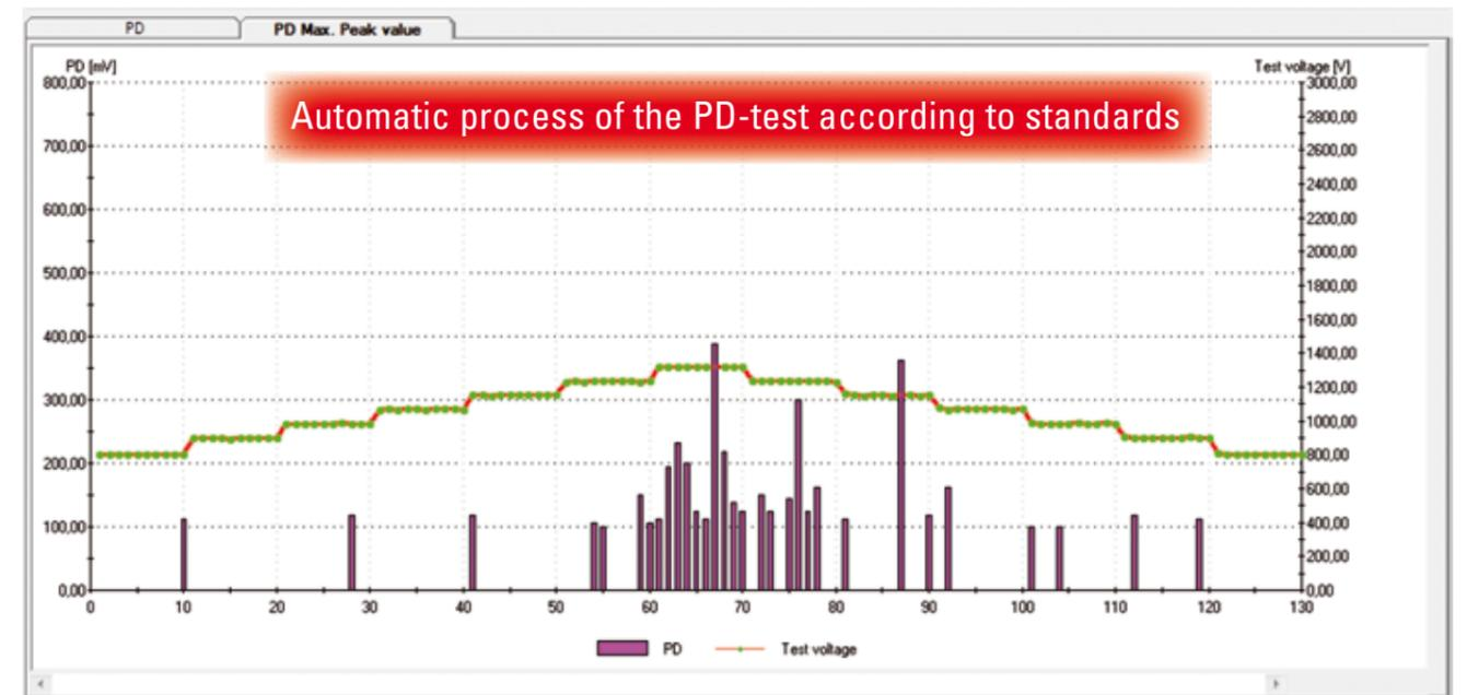
The test is performed either manually or automatically. In the manual mode the operator increases the voltage continuously while monitoring the partial discharge signal. Via a test sequence the automatic operation provides an analysis of all three phases. The following values are determined per phase:
