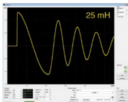
The inductance is calculated from the surge voltage test's signal. The result is indicated in "H".
