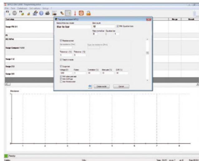
The armature assistant is a tool to create test programs. After entering the required data (quantity bars, test voltage, etc.) a corresponding test plan is generated.
