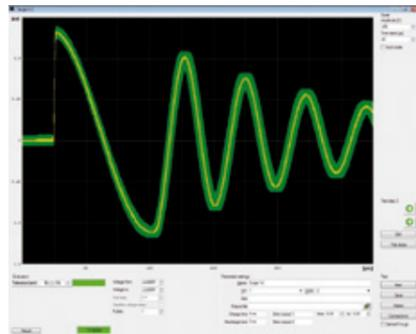
The tolerance band belongs to the simpler evaluation methods, at which an envelope curve is placed around the signal. The surge wave has to be within a certain tolerance band.
