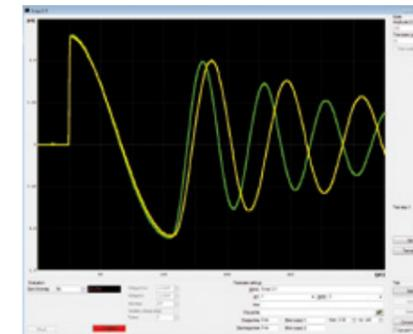
The difference in frequency between reference surge wave and currently measured surge wave is automatically determined and the deviation is indicated in %.
