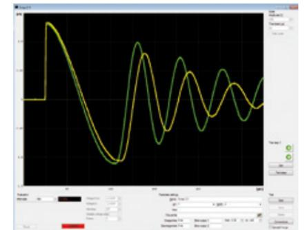
The difference in the attenuation course between reference surge wave and currently measured surge wave is automatically determined and the deviation is indicated in %.
