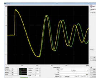
The comparison to a reference is possible, in case a good test object has been taught-in before. Normally this method is used in production.
