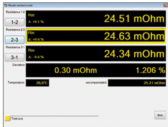
Resistance test at a 3-phase machine
