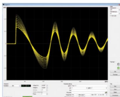
At the peak-to-peak-method the test voltage is gradually increased. If a bigger deviation occurs between two steps, the test is stopped. The deviation from step to step is indicated in %.
