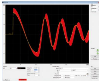
The error area is the differential area between 2 signals (surge waves). The difference in area between reference surge wave and currently measured surge wave is automatically determined and the deviation is indicated in %.
