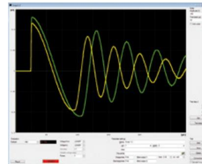
The relation between reference surge wave and currently measured surge wave is automatically determined and the deviation is indicated in %.
