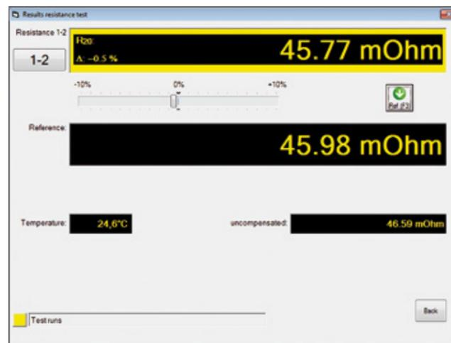
Resistance test e.g. at an air-core coil or bar-to-bar
