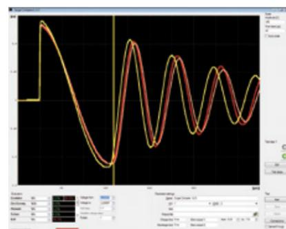
At the phase comparison all three phases of a motor are automatically compared with each other and displayed in a diagram. In this way the symmetry can be directly determined and evaluated. Normally this method is used in the motor repair sector.
