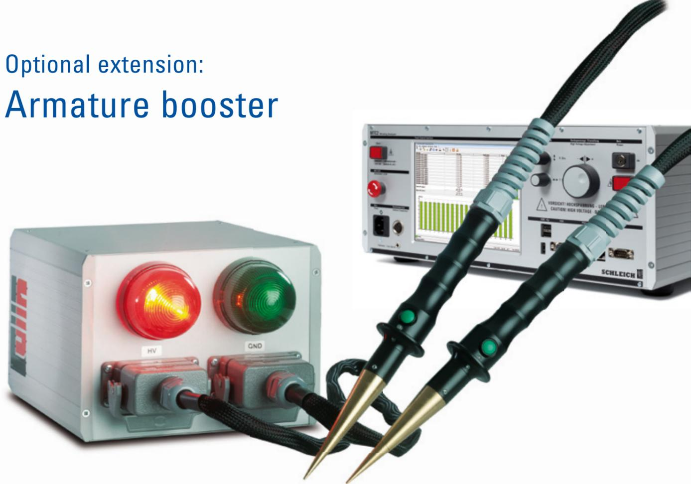
For the armature test an additional armature booster is available for MTC2-testers. This is necessary for testing of larger, low-inductive DC-armatures. With the armature booster the surge current is increased by factor 10, to find short-circuits and insulation faults between bars.
