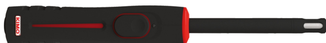
Hygrometry probe* Measuring ranges from 3 to 98%RH, from -50 to +100 °Ctd and -20 to +80°C
