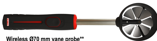
Wireless Ø70 mm vane probe** Measuring ranges from -5 to 35 m/s, from 0 to 99999 m 3 /h and from -20 to +80 °C
